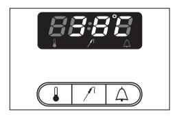
the actual core temperature appears in the oven display. N.B. The lowest temperature that can be displayed is 20°C, so this will also be shown until the roast probe registers 20°C.
